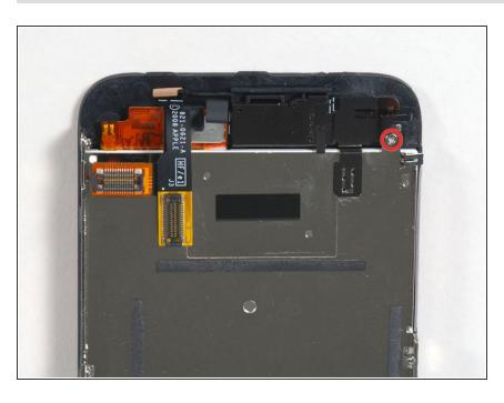
Remove the single Phillips #00 screw from the corner of the display assembly.
