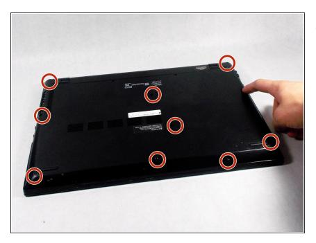
Unscrew the 10 9.0 mm screws holding the back panel on using a Phillips head #1 screwdriver.
