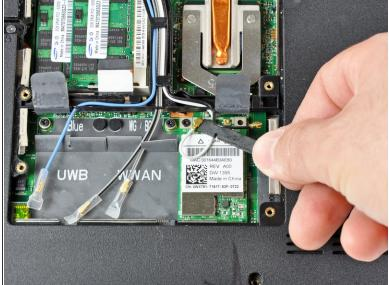
Use the flat end of a spudger to gently pry the black and white antenna connectors off the Wireless Mini-Card.
