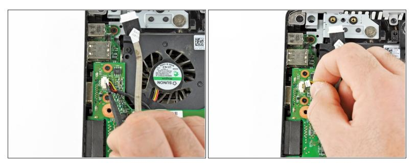
• Disconnect the fan cable connector by pulling it towards the fan with a spudger.
