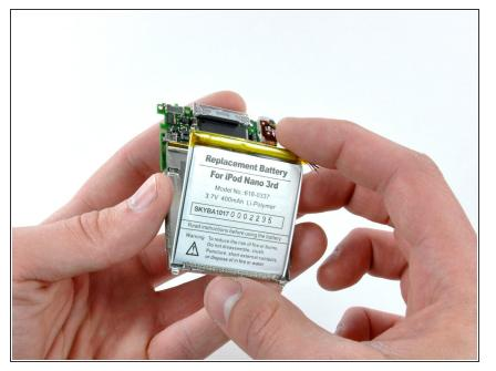
Place the new battery in the metal battery tray, sticking it down to the adhesive.
