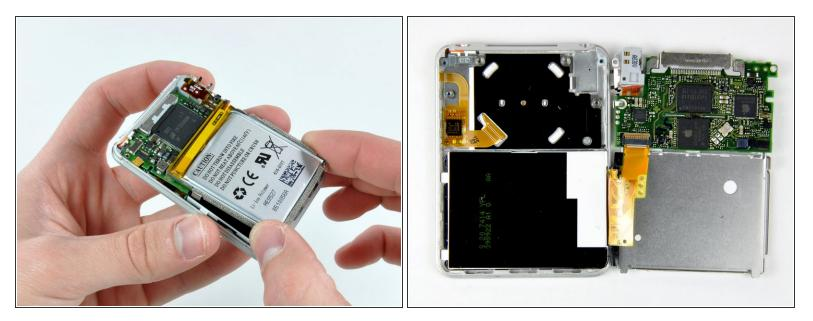
▲ The logic board is still connected to the front case by the display ribbon cable, located on the headphone jack side of the logic board.
