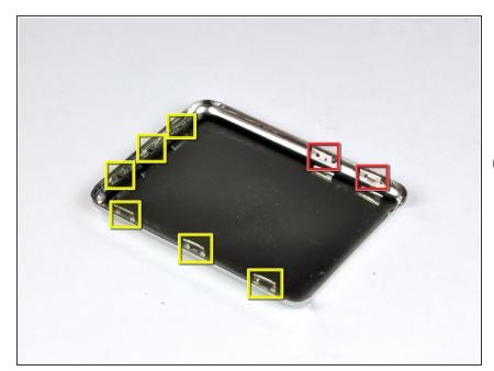
The rear panel is secured to the front case by eight clips permanently attached to the rear
