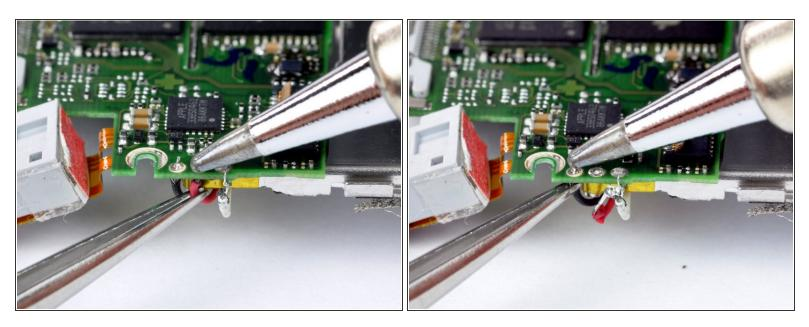
• De-solder the remaining leads, following the procedure illustrated in the previous step.
