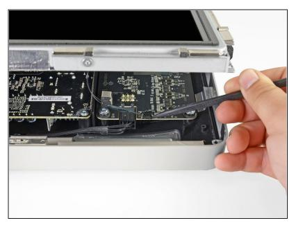
Disconnect the vertical sync cable in the upper left corner of the screen. Use the tip of a spudger to push on the connector's side tabs and gently walk it out of its socket.
