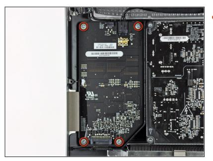
Remove the four T10 Torx screws securing the LED driver board to the outer case.
