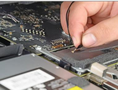
Pull the black tab straight up to disconnect the latch on the display data cable ZIF connector.
