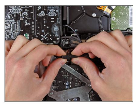
Disconnect the AC power inlet cable by depressing the locking mechanism while pulling the connector away from its socket.
