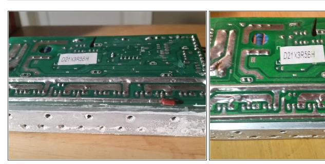
Notice the thick lines of solder on the board especially - this helps the power flow without burning out thin lines- this is an impressive controller on a cheap bike so far!
