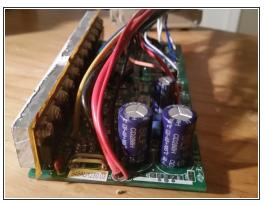
Remove screws, loosen white plastic screw, slide casing end over wires to expose & remove controller. Look for any signs of water or overheat damages. In pic 3 notice the red wire and on the board next to it are two pieces what appears to be bare wires. They are shunts & can be soldered a bit on ends to add output power. DON'T solder all the way!!
