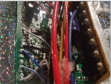
• Inspect controller insides for broken wires and swelled capacitors and frayed wires loose solder points on the board. 2nd pic looks like the board is wet- normally a bad thing I have a new spray that protects it. Get to that later. I can smell burnt parts at times. Sniff around for the stinky electronic smell for clues and brown/black Hot spots!
