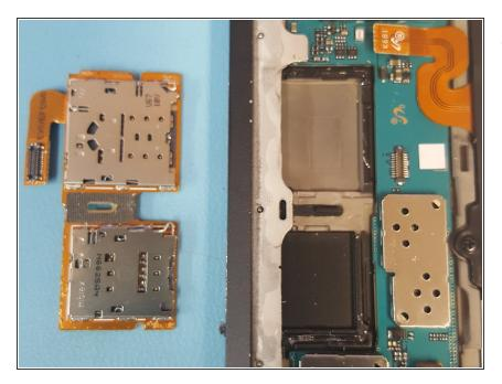
Disconnect the SIM card reader flex cable as well, and then carefully pry the SIM card/microSD card reader out.
