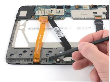
• Use the flat end of a plastic spudger to gently pry the press-fit connector from the microphone's ribbon cable.
