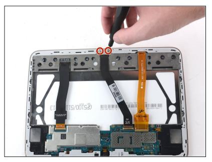
Use a Phillips #000 screwdriver to remove the two 3mm screws in the metal plate connecting the charging port to the display assembly.
