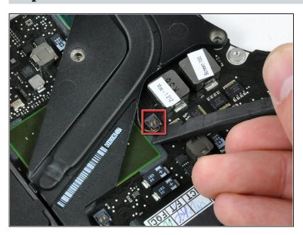
Use the flat end of a spudger to pry the thermal sensor connector up off the logic board.
