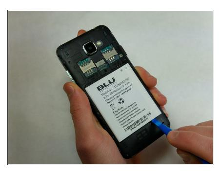
Pry the battery out using the plastic opening tool.
