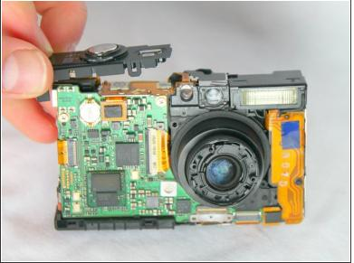
Using the spudger, take off the shutter button by prying the small tab on the front side of the camera.
