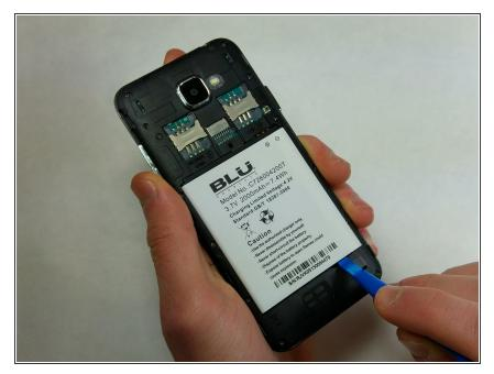
Pry the battery out from the back of the phone using the plastic opening tool.
