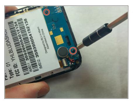
Unscrew the 2.5mm screws from the circuit board holding the speaker at the bottom of the phone.
