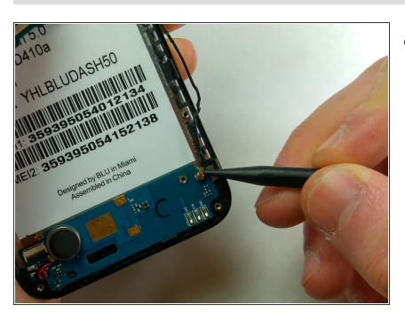
Remove the antenna cable connectors using a spudger.
