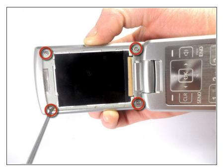
Unscrew the four corner 3.21mm screws to separate the top cover of the phone
