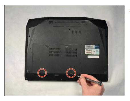
Flip the laptop over and remove the two 4mm screws located at the bottom of the laptop with the PH0 screwdriver.
