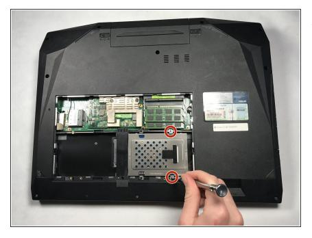
Locate the two, 4mm screws on the hard drive. Remove them with the PH0 screwdriver.
