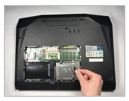
• Using the black tab located on the hard drive, pull out the hard drive.
