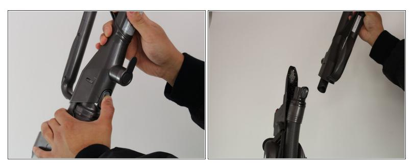
• With the vacuum placed upright, press firmly on the gray button, located on the back of the handle, and pull directly upwards until handle is completely removed from the rest of the vacuum
