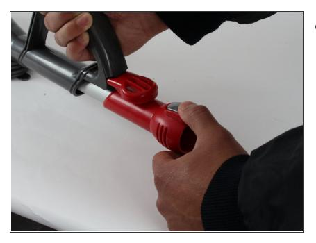
• Pull the nozzle until it is completely out of its housing.
