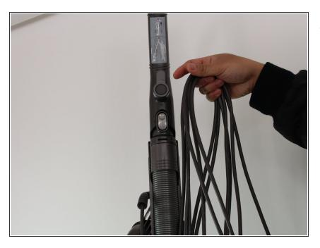
• Begin by completely unwinding the wire on the back.
