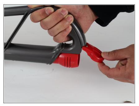
• Place the vacuum either upright or on its back and lift the nozzle lid to access the nozzle.
