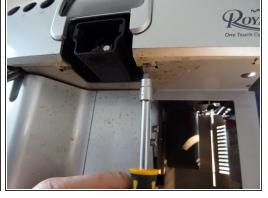
• The screws are situated on the underneath of the cover. This type is held by four screws.
