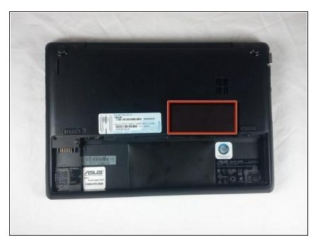
With the battery removed, locate the RAM cover.
