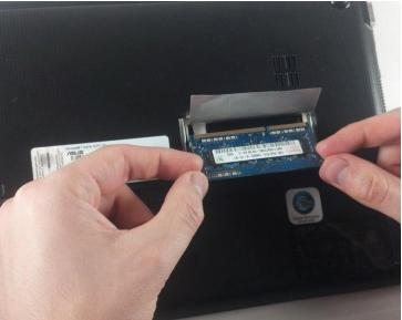
• Carefully grasping the edges of the RAM module, slowly pull it free from the pin connectors underneath the edge of the foil.
