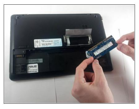
Remove RAM module entirely for repair or replacement. To reassemble your device, follow these instructions in reverse order.
