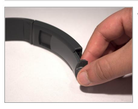
Using a little amount of force, slide the plastic cover off of the headband.
