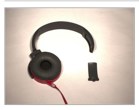
Pull the plastic until the cover is fully removed.
