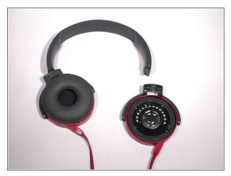
With the swivel screw removed, remove the plastic casing.
