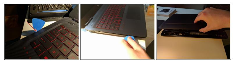
$\bigwedge$  The laptop scratches easily, be careful when removing the back cover.
