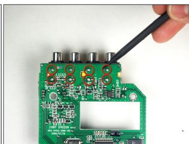
• On the circuit board with the AVI Port, de-solder the circled areas on the back to remove the AVI Port.
