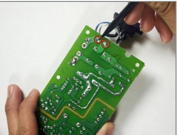
• On the circuit board with the Power Port, de-solder the circled areas on the back to remove the Power port.
