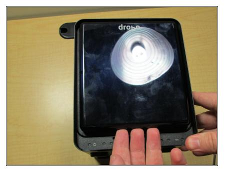
• Place fingers under front panel and pull up and away to remove it.
