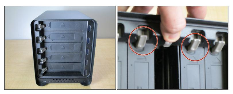
Depress tabs on side of front panel and slide hard drive out.
