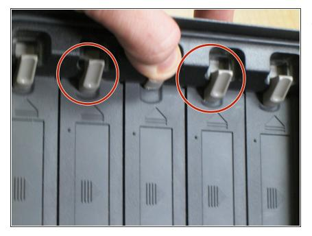
To replace hard drive, depress tab on an empty slot and slide hard drive in. Making sure to align the drive ports with connectors in the back of the drive slot.
