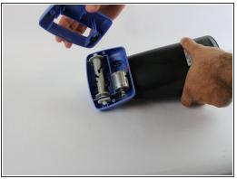
Once the screws are removed pull the front face plate off. This will allow access to the belt and motor.
