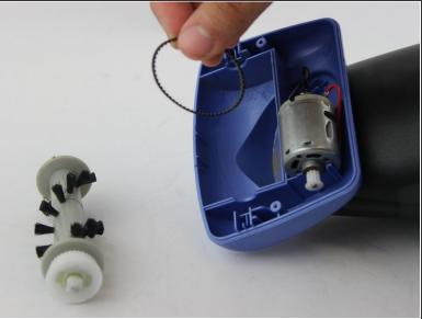
• Remove the belt from the motor mount, and then replace with a new belt.
