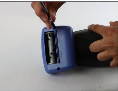
Remove the two 12mm screws from the front face plate with the PH2 bit from the tool kit.
