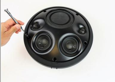
Remove the five 14.4 mm T10 Torx screws.
