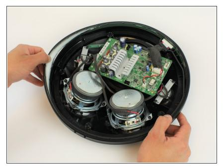
Pull the silicone button band off of the outer edge of the speaker.
