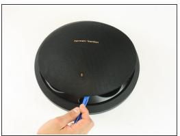
Using a plastic opening tool, pry off the front grill by wedging it in the notch on the front of the device.
