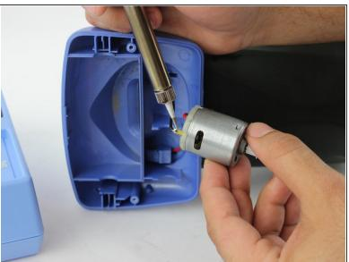
Remove the solder from both motor terminals.
