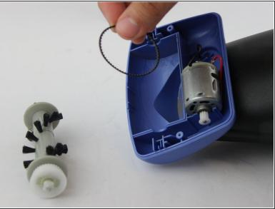
• Remove the belt from the motor mount, and then replace with a new belt.
