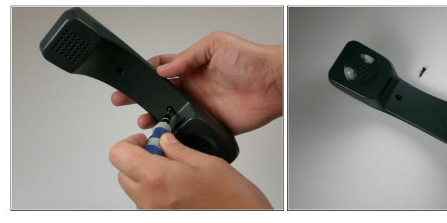
Unscrew the two black screws (8 mm long) located in the middle of the handset using #1 Phillips head.
