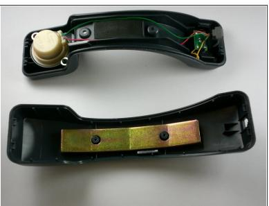
Pry the back cover off the headset using a spudger. It is best to pry at the top of the handset.
