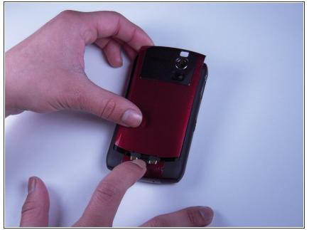
Press down on the battery release button and slide the back cover up with your thumb.
