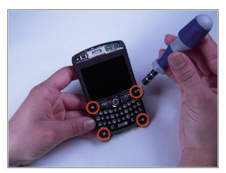
Remove the four T6 Torx screws located on the corners of the keyboard frame.
