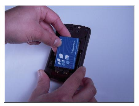
• Pry from the top of the battery to pull it out.
