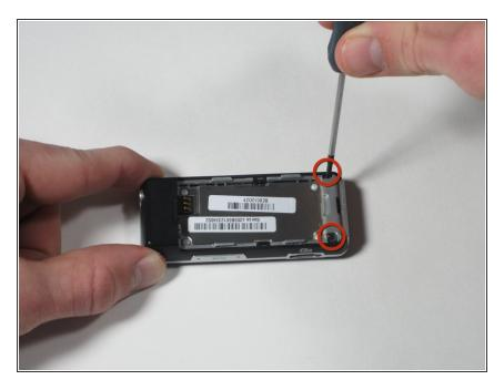
Remove the two black .265" screws at the base of the device.
