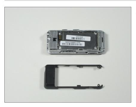
The rear case cover can now be separated from the device.
