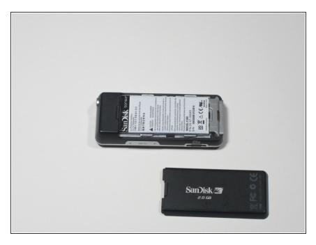
The back cover is now separated from the device.
