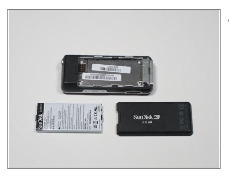
The battery is now removed from the device.
