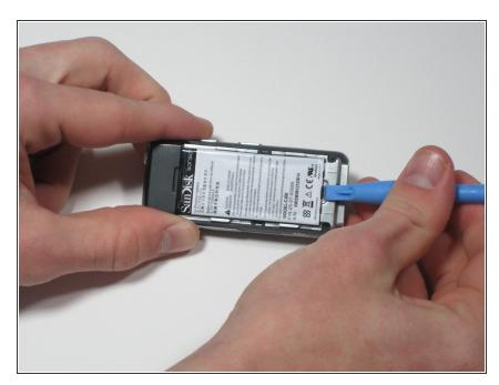
Apply a fingernail or a plastic opening tool to the base of the battery.
