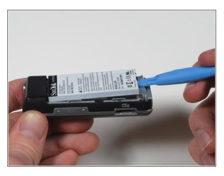
Lift up gently. The battery should come up and out.
