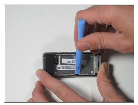
Using a plastic opening tool, pry up the two arms of the case cover near the middle of the device to free them from the sides.
