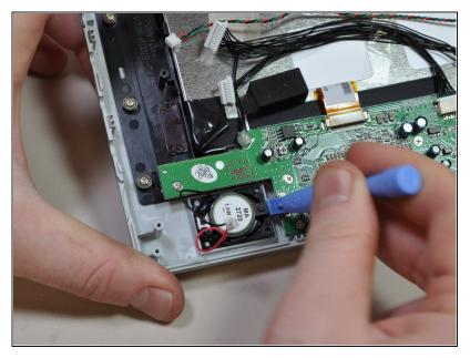
Use a plastic opening tool to lift the speaker(s) free of the retaining posts.
