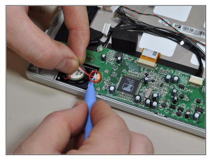
Disconnect the speaker wire(s) from the logic board.
