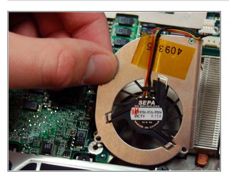
Lift the cooling fan out of the laptop.
