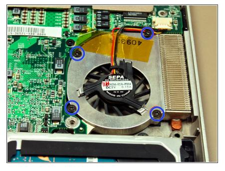
Remove the 4 3 mm screws that hold the cooling fan to the system board.
