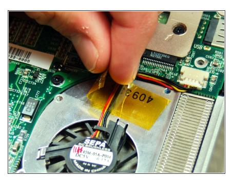
Remove the tape holding the cooling fan wires down.
