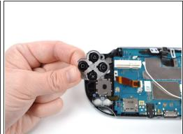
Using tweezers, gently peel the action button off the back casing assembly.
