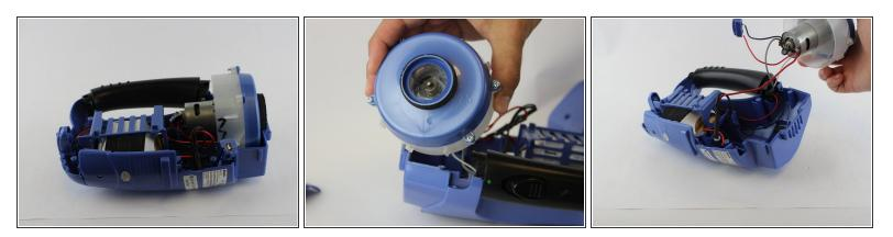
• Pull the motor upward and away from the the housing.
