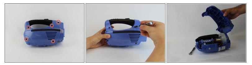
• Remove the five 14mm screws with the PH2 Bit from the motor housing and pull the housing apart.
