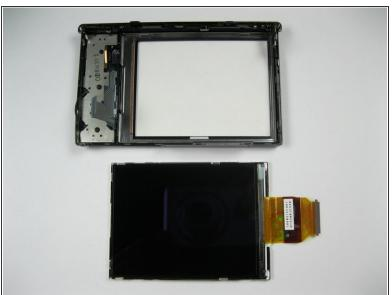
Pry the display from the rear casing using a spudger.
