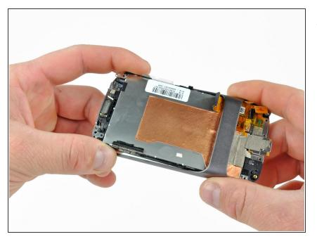
• Pull up on the screen so it slides out of the case.
