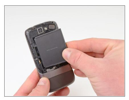
• Pull the battery up and out.
