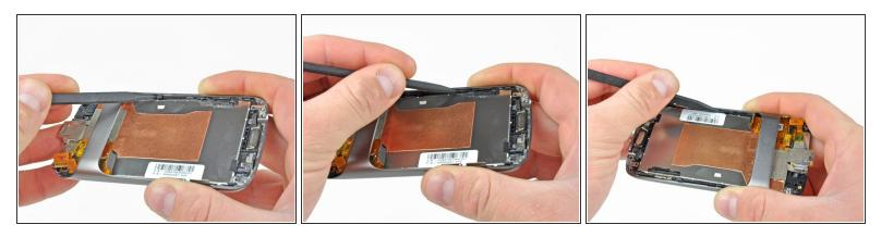
• Use the spudger to pop the 3 latches holding the screen down.
