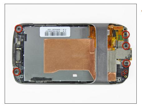
Remove the seven #00 Philips screws
