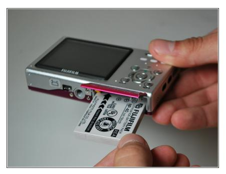
Insert the new battery and close the battery cover.
