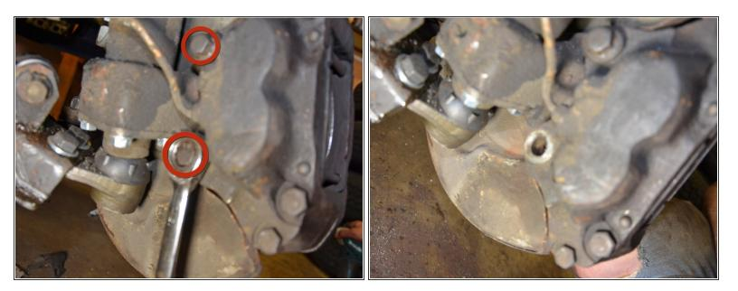
Use a 15 mm box end wrench to remove the two bolts on the back of the brake caliper.
