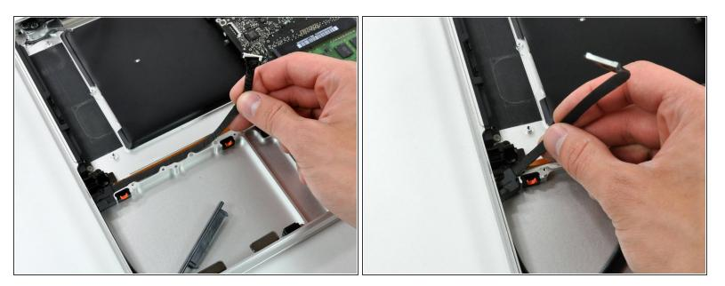
Peel the hard drive cable from the adhesive securing it to the upper case, and maneuver the plastic retaining block out of the upper case.
