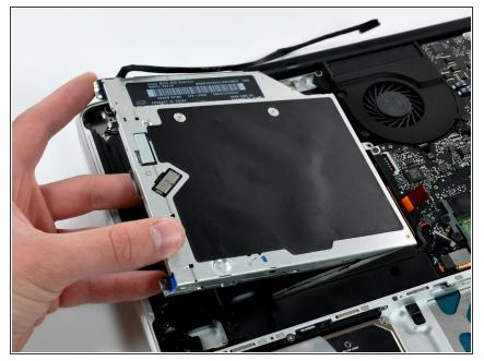
• Lift the optical drive from its left edge and pull it out of the computer.
