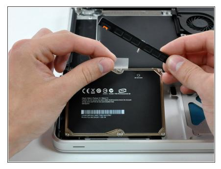
• Lift the hard drive by its plastic pull tab and remove the freed hard drive bracket.
