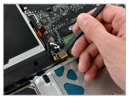
• Use a spudger to pry the trackpad connector straight up out of its socket on the logic board.
