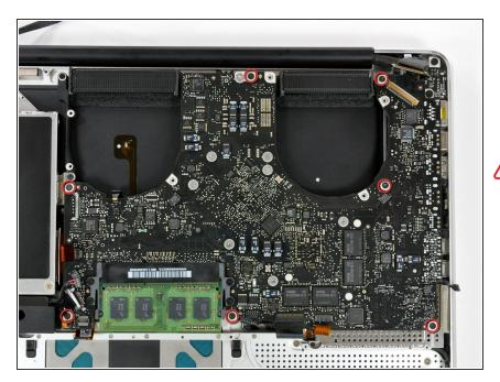
Remove seven 3.2 mm Phillips screws securing the logic board to the upper case.
