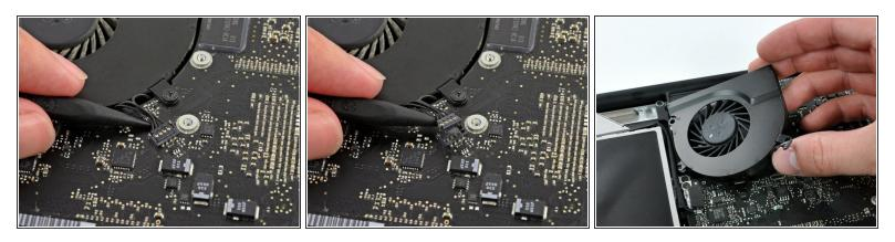
Use the tip of a spudger to lift the right fan connector straight up from its socket on the logic board.
