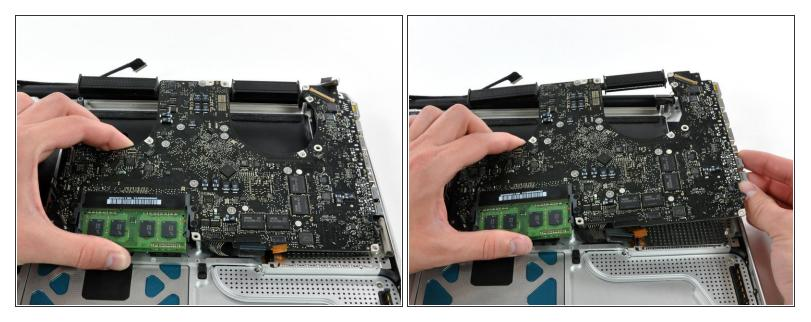
• Carefully lift the logic board assembly from the left side and work it out of the upper case, minding the port side that may get caught during removal.
