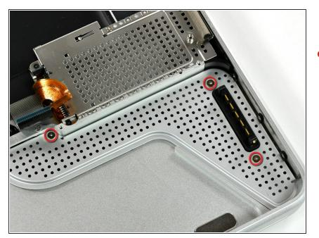
Remove three 2 mm Phillips screws securing the battery connector cover to the upper case.
