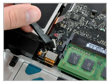
Use the flat end of a spudger to pry the silver-colored hard drive cable connector straight up out of its socket on the logic board.
