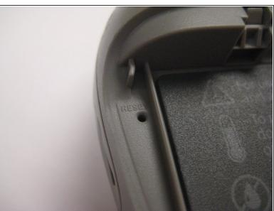
After removing the battery cover and battery, locate the reset (indicated by arrow).
