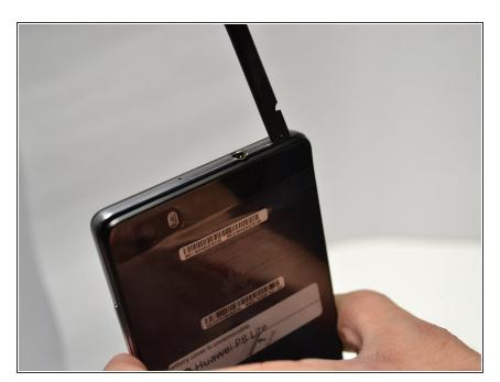
• Then remove the back cover of the device with the <u>Spudger</u>. To prevent damage to the back cover, begin removing the cover half an inch to the right of the headphone jack and continue prying around the perimeter of the device.
