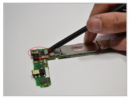
Once the motherboard is removed use the <u>Spudger</u> to remove the Front Camera.
