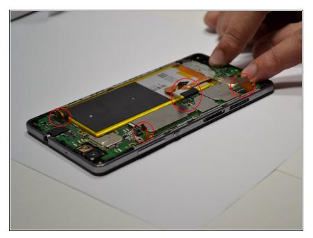
• Gently separate the connectors attached to the motherboard.
