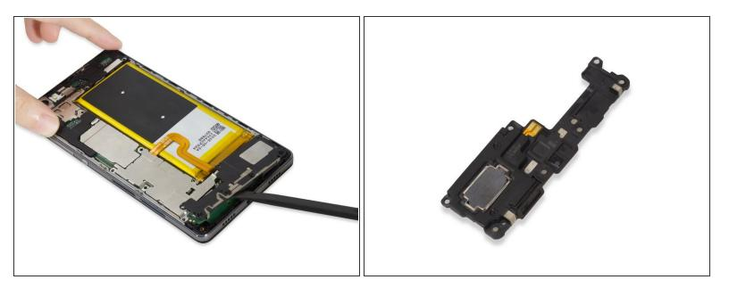
Use the <u>Spudger</u> to gently remove the Loudspeaker from the device. Place the replacement Loudspeaker into the device and follow these steps in reverse order to reassemble the device.
