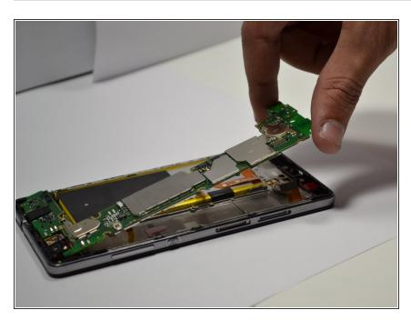
• Carefully remove the motherboard from the device.
