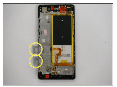
Using the <u>Spudger</u>, begin by removing both of the SIM slots from the side of the device.
