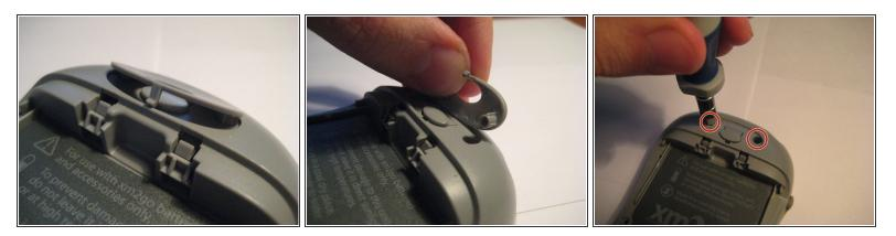
• Remove the two screws under the button using the T6 Torx screwdriver.
