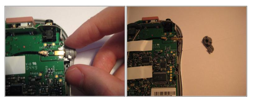
• Remove the plastic antenna extension connector on the right side of the device.
