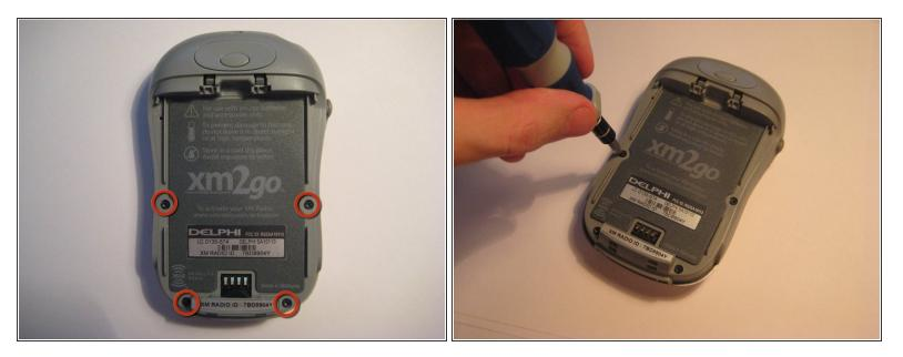
• Remove the four screws from the bottom of the device using a T6 Torx screwdriver.
