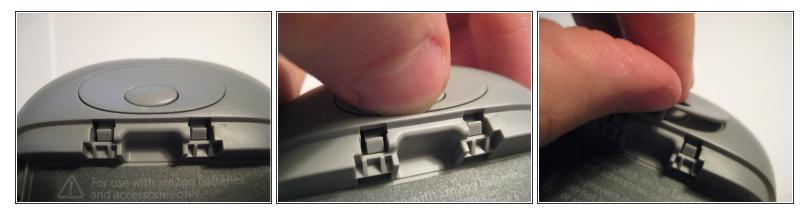
Remove the button cover on the back of the device by prying it up with a spudger or your thumb nail.
