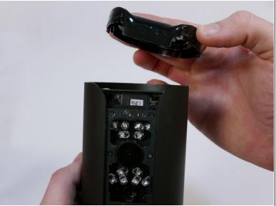
Pull the top casing away from the device.
