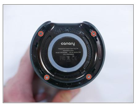
Use your Phillips #0 screwdriver to remove the four 6mm screws.
