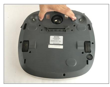
Press and hold the tabs on both sides of the battery.
