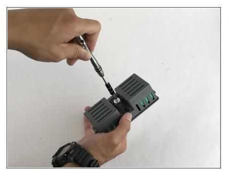
• Remove the screw attaching the battery housing.
