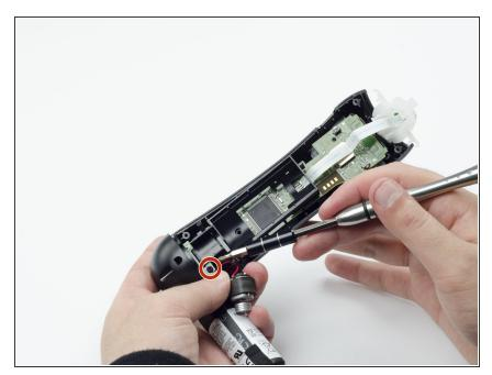
Unscrew the 9mm screw behind the rumble motor slot with a PH #00 screwdriver.
