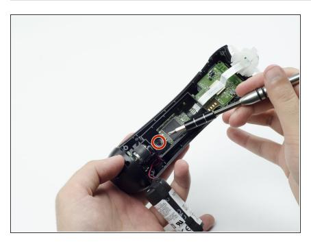
Unscrew the 9mm screw in the battery slot with a PH #00 screwdriver.
