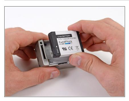
Remove the battery from the case.
