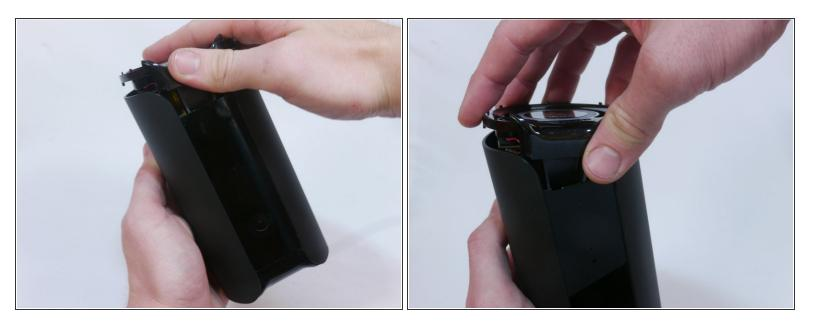
↑ Do not yank the bottom off or you may damage the ribbon cable or the ZIF connector.
