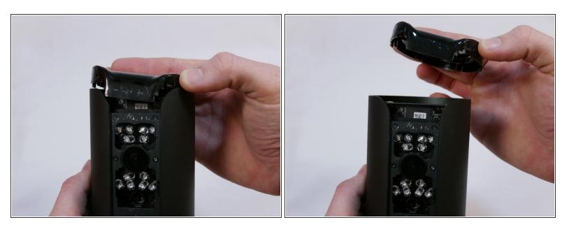
• Pull the top casing away from the device.
