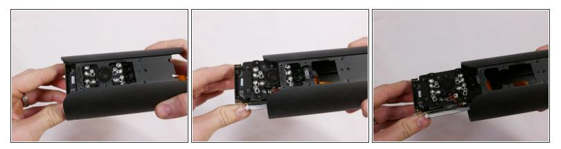
• Grip the circular part of the motherboard and pull it straight out of the device.
