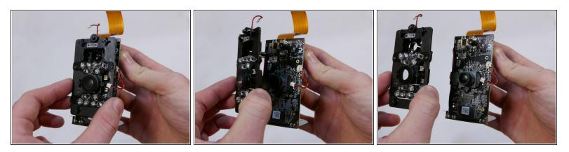
• Lift the infrared LED board directly upwards and pull away from the motherboard.
