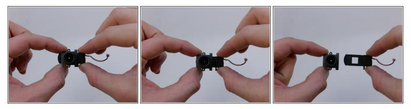
• Grab the battery end of the filter and pull to slide it out.
