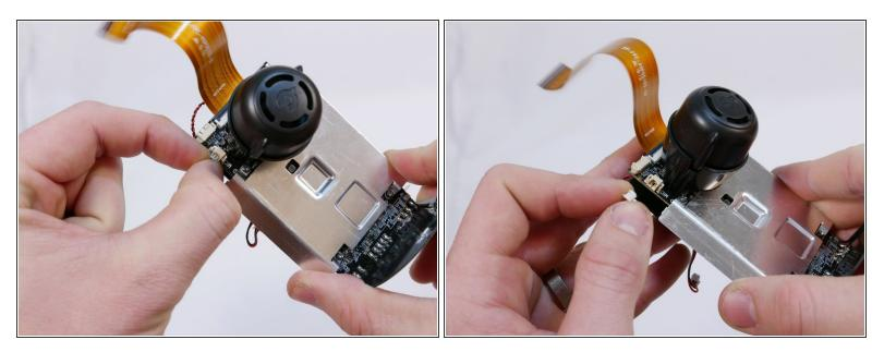
• Find the power connector next to the buzzer that is labelled "MIC IR-LED". Use your fingers to wiggle it back and forth until it becomes loose.
