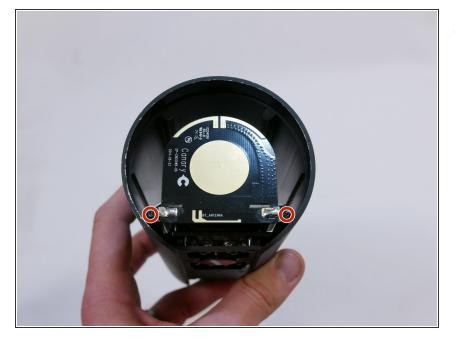
• Use your Phillips #0 screwdriver to remove the two 5mm screws.
