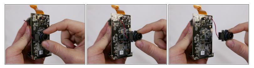
Using your forefinger and thumb, grip the top and bottom of the lens assembly and pull away from the motherboard.
