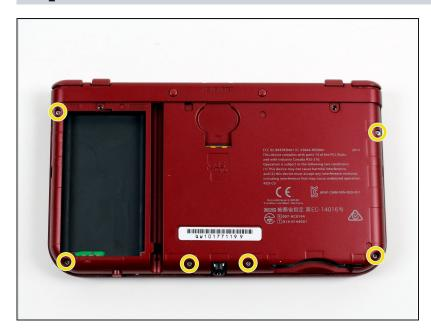
Using a JIS #000 screwdriver, remove the six 6mm screws around the edges of the secondary cover.
