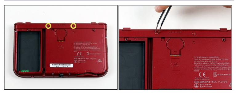
Using tweezers, carefully pop out the rubber bumpers located at the top side of the 3DS. Removing them will reveal another two 6mm screws. Remove these screws using a JIS #000 as well.
