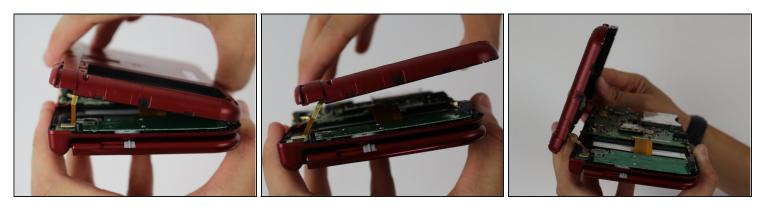
• To separate the cover, carefully lift it up and away from the hinges (in order to clear the headphone port), then pivot it towards the hinges to expose the circuit boards.
