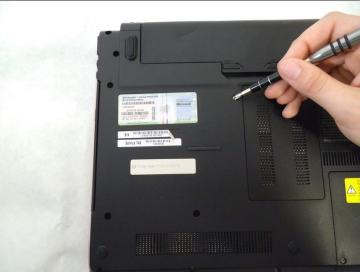
• Remove the four 5.2mm screws that are holding in the Disc Drive.
