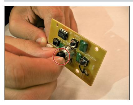
Turn the knob on the circuit board left or right to adjust the browning dial.
