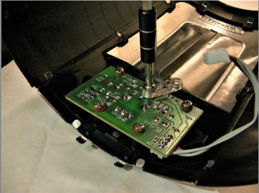
• Unscrew the circuit behind the browning dial on the front cover.
